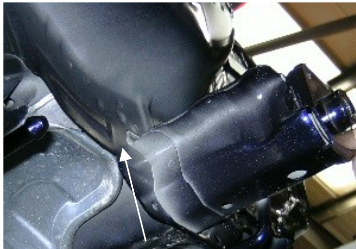
DRILL OUT SPOT WELD AT POSITION SHOWN AND FIX WITH BOLT (P)
