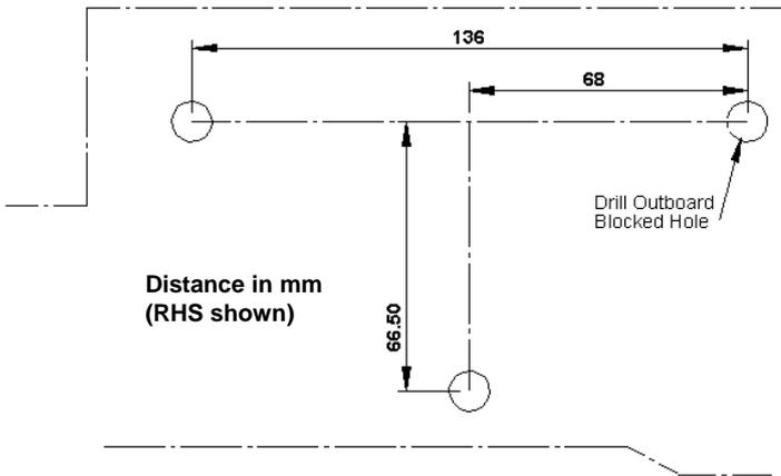
For blocked outboard holes, mark distances accurately. Drill small pilot hole, and then open hole with cone cutter to prevent damage to threads
