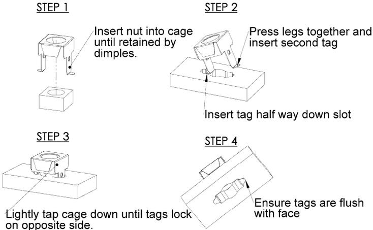
Inserting Caged Nut into closed hole (e.g. end of cross tube)
