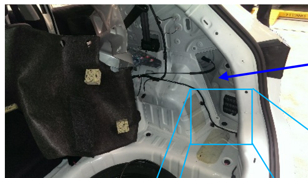
The TF2218/7PIN, TFC2 and TFR1, are to be secured to the car in this area.
