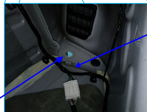
Access to MG towing Connector on car loom, Towing module and relay Module's housed here,
